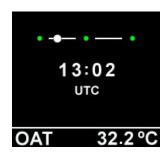
Displays UTC time, seconds on the minute progress bar and the Outside Air Temperature at the bottom of the instrument.
