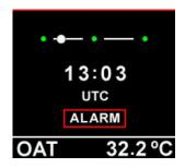
When an external alarm input is sensed the annunciator is active and the ALARM notification will be displayed on the current screen.
