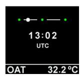
Displays UTC time, seconds on the minute progress bar and the Outside Air Temperature at the bottom of the instrument.
