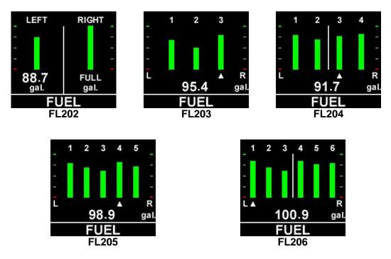
For the FL202 instrument, the quantity in each tank is permanently displayed beneath each indicator bar. For all other instruments, use the bottom button to scroll between tanks. The fuel quantity displayed corresponds to the tank number with the arrow beneath the bar indicator.
