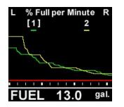
This screen provides a graphical display of fuel usage, since the most recent power on.
