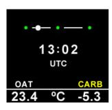
The CARB label on the bottom of the screen will turn yellow when carburetor air temperatures are in the potential carb icing zone.
