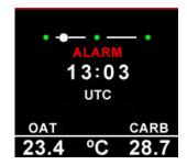
When an external alarm input is sensed the annunciator is active and the ALARM notification will be displayed on the current screen.
