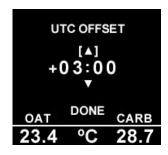
To change or set the UTC offset, press the bottom button and follow the onscreen instructions to set the offset. Use the bottom button to navigate and the top button to set.
