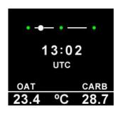
Displays UTC time and seconds on the minute progress bar. The Outside Air Temperature and Carburetor Air Temperature are at the bottom of the instrument.
