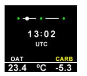
The CARB label on the bottom of the screen will turn yellow when carburetor air temperatures are in the potential carb icing zone.
