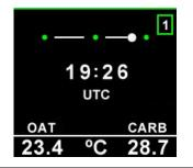
At the time of the interval period, the interval timer notification will be displayed on the top right in a green box. The value in the box is the minute value of the interval.
