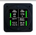
Oil pressure and temperature, voltmeter and ammeter systems
