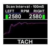
This screen provides a graphical display of left and right engine RPM.
