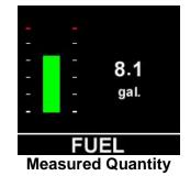
The quantity in the tank is digitally displayed to the right of the indicator bar.
