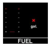
FUEL INSTRUMENT NOT INSTALLED CORRECTLY FLIGHT PROHIBITED
