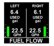
Displays the total fuel used, for each engine, since the instrument was last restarted, on the top portion of the display. **NOTE: Each time the instrument restarts the "USED" amount is reset to zero.**
