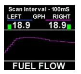
This screen provides a graphical display of the fuel flow for both left and right engines
