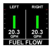
Displays the fuel flow for both left and right engines. Colors are determined by the range values as set during installation.
