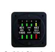
Four Cylinder Exhaust Gas and Cylinder Head Temperature
