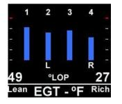
The cylinder with the "R" letter beneath it is the richest cylinder and the "L", the leanest.
