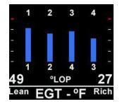
Press the bottom button to view the order in which the cylinders peaked.
