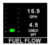
Displays the fuel flow and total fuel used for the engine. Colors are determined by the range values as set during installation.
