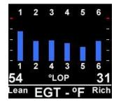
All cylinder conditions (LOP) will be between the values of the lean and rich temperatures. Your engine mixture has now been set to the desired LOP value.
