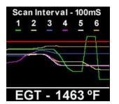
The temperature displayed is that of the hottest cylinder.
