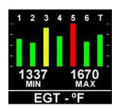
Turbine Inlet Temperature is not included in MIN and MAX temperature values or a function of the leaning process. It is a display only parameter.
