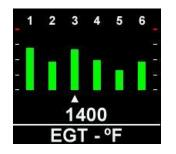
Use the bottom button to scroll to the desired cylinder (default is 1).
