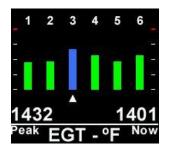
The first cylinder to peak will be displayed in blue with an arrow beneath it. **STOP LEANING.**
