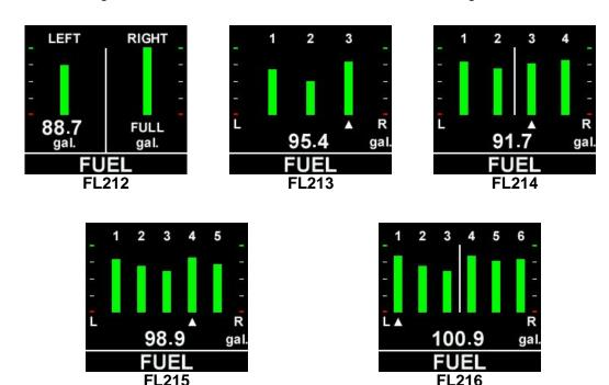
For the FL212 instrument, the quantity in each tank is permanently displayed beneath each indicator bar. For all other instruments, use the bottom button to scroll between tanks. The fuel quantity displayed corresponds to the tank number with the arrow beneath the bar indicator.
