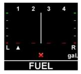
FUEL INSTRUMENT NOT INSTALLED CORRECTLY FLIGHT PROHIBITED
