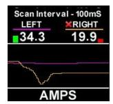
This screen provides a graphical display of the current flow information for both current sources.
