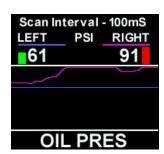
This screen displays the oil pressure, for both left and right engines, graphically.
