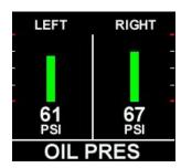
Displays the oil pressure, for both left and right engines. Colors are determined by the range values as set during installation.
