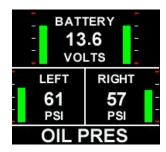
Displays the battery voltage on the top half of the display and the oil pressure on the bottom half.
