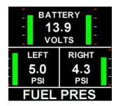
Displays the battery voltage on the top half of the display and the fuel pressure on the bottom half.
