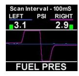
This screen displays the fuel pressure for both left and right engines.
