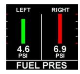
Displays the fuel pressure, for both left and right engines. Colors are determined by the range values as set during installation.
