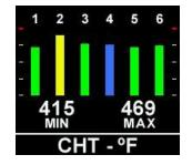
If the temperature of one or more cylinders changes by an amount greater than the preset shock cooling value, then the specific cylinder indication will turn blue and flash.
