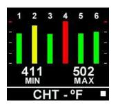
Displays the temperature of all cylinders in a graphic format. Colors are determined by the values set during installation.
