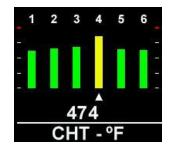
Use the bottom button to scroll to the desired cylinder (default is 1).
