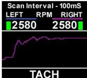
This screen provides a graphical display of left and right engine RPM.
