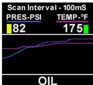
This screen displays the oil pressure and temperature graphically.
