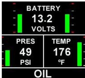
Displays the battery voltage on the top half of the display and the oil pressure and temperature on the bottom half.
