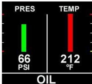
Displays the oil pressure and temperature. Colors are determined by the range values as set during installation.
